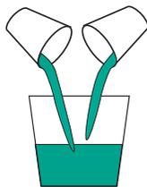
Transfer mixture to **CLEAN MIXING CONTAINER #2** and mix thoroughly using your stir stick to scrape the sides and bottom. Once completed, apply immediately.
